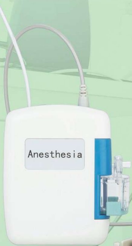
Standard CO 2 , N 2 O, ISO, SEV, DES, HAL, ENF, Optional for paramagnetic O 2
